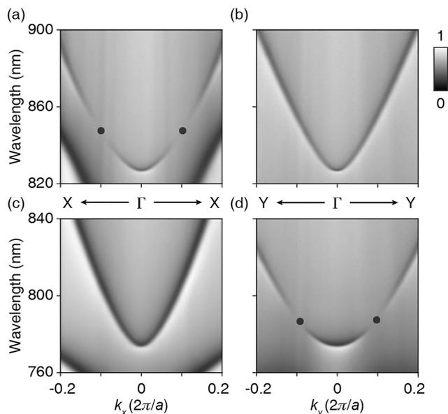
**Figure 2.** Measured angle-resolved transmittance spectra of the PhC slabs with  $C_2$  symmetry. The black dots correspond to the off- $\Gamma$  BICs. (a,b) The spectra of the  $t = -0.06$  sample under  $s$ -polarized incidence (a) and  $p$ -polarized incidence (b). (c,d) The spectra of the  $t = 0.06$  sample under  $s$ -polarized incidence (c) and under  $p$ -polarized incidence (d).
